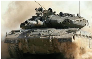
Figure 18 The Merkava tank and other military vehicles employ KVH DSP FOGs for turret stabilization
